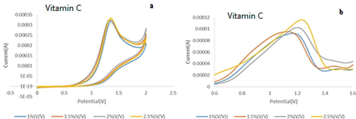
**Fig. 5. a:** Cyclic voltammetry of ascorbic acid **b:** Square Wave voltammetry of ascorbic acid.
