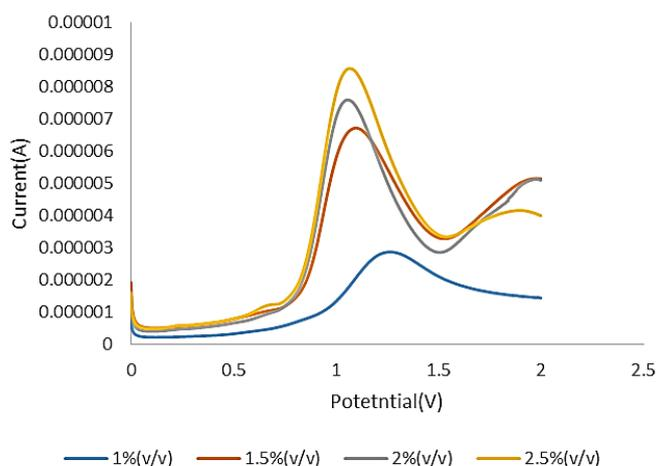
**Fig.4.** Square wave voltammetry of *Thymus* in different concentrations. Potential was swept between 0 and 2.0 V. pH was set at 3.0.
