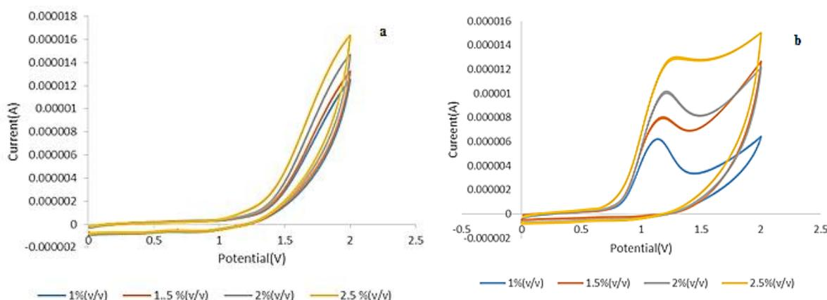
**Fig. 3.** Cyclic voltammetry of **a:** *Thymus*, **b:** *Thymus* after spike Potential was swept between 0 and 2.0 V. Scan rate was  $0.1 \text{ Vs}^{-1}$ . pH was set at 3.0. Cathodic peak current ( $I_{pc}$ ) increased with the increment thymol concentration.
