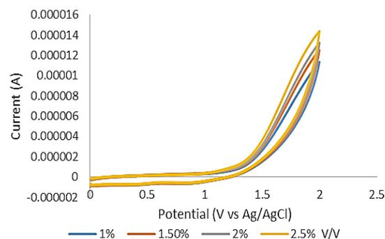
**Fig. 3.** Cyclic voltammetry of *Ajwain*; Experimental conditions: pH= 3.0,  $v = 0.1 \text{ Vs}^{-1}$  in different concentration, potential = 0 to 2.0 V, temperature = 25 °C.
