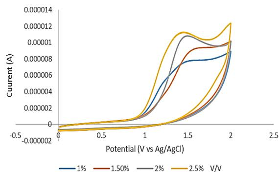
**Fig 4.** Cyclic voltammetry of *Ajwain* after spike; Experimental conditions: pH= 3.0,  $v = 0.1 \text{ Vs}^{-1}$  in different concentration, potential = 0 to 2.0 V, temperature = 25 °C, The cathodic peak current ( $I_{pc}$ ) increased with the increment thymol concentration.
