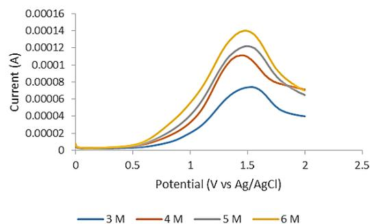
**Fig. 7.** Square wave voltammograms of pure thymol for calibration, Experimental conditions: pH= 3, potential = 0 to 2.0 V, temperature = 25 °C.
