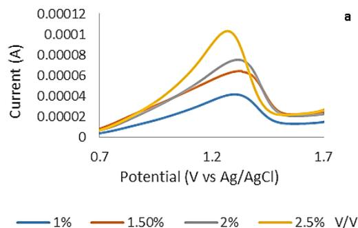
**Fig. 6. a:** Cyclic voltammetry of Ascorbic Acid, b: square wave voltammograms of Ascorbic Acid; The anodic peak currents ( $I_{pc}$ ) vividly increased in the square wave voltammograms compared to the Cyclic voltammetry; Experimental conditions: pH= 3.0 in different concentration, potential = 0 to 2.0 V, temperature = 25 °C.
