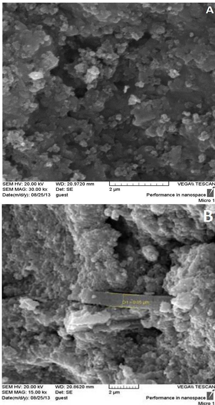
**Fig. 3.** SEM image of SnO<sub>2</sub> (A) and C,N,S-tridoped SnO<sub>2</sub> (B) nanoparticles.
