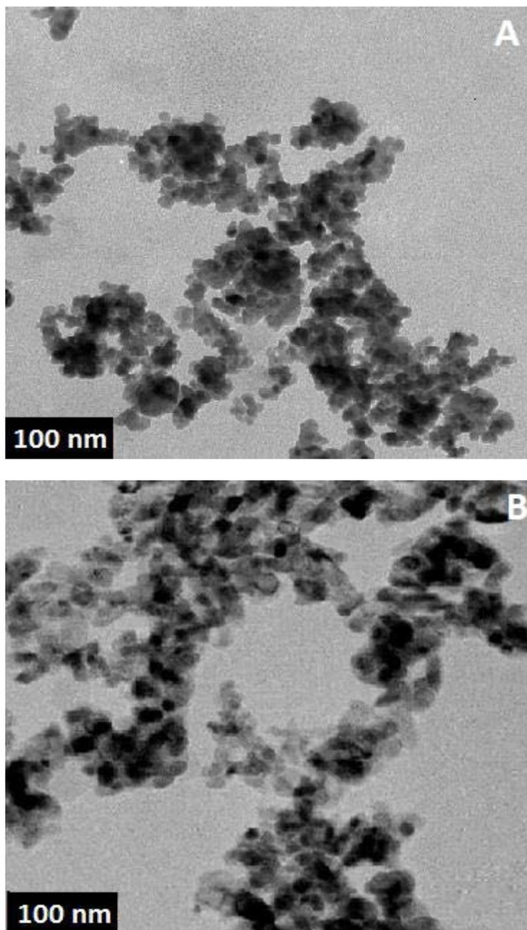
**Fig. 4.** TEM image of SnO<sub>2</sub> (A) and C,N,S-tridoped SnO<sub>2</sub> (B) nanoparticles.
