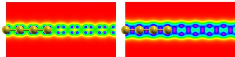
**Fig. 5.** A simulated STM image of Au-LC is obtained from DFT (left) and DFT +U (right).
