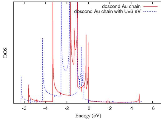
**Fig. 8.** DOS of Au liner chain within DFT and DFT+U calculations. Fermi level is set to zero.
