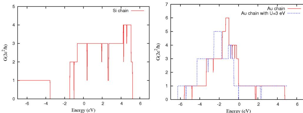
**Fig. 6.** Calculated quantum conductance of Si and Au liner chains in terms of bias voltage. Fermi level is set to zero.
