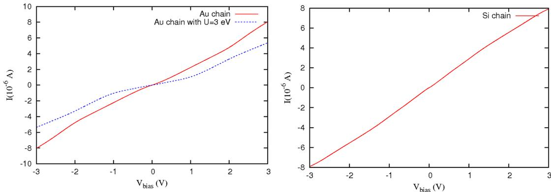
**Fig. 9.** I-V curve of Au and Si liner chains in terms of bias voltage. Fermi level is set to zero.
