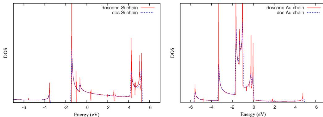
**Fig. 7.** DOS and DOScond of Au and Si liner chains. Fermi level is set to zero.
