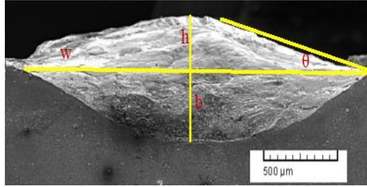
**Fig. 1.** Geometrical features of a laser clad track.
