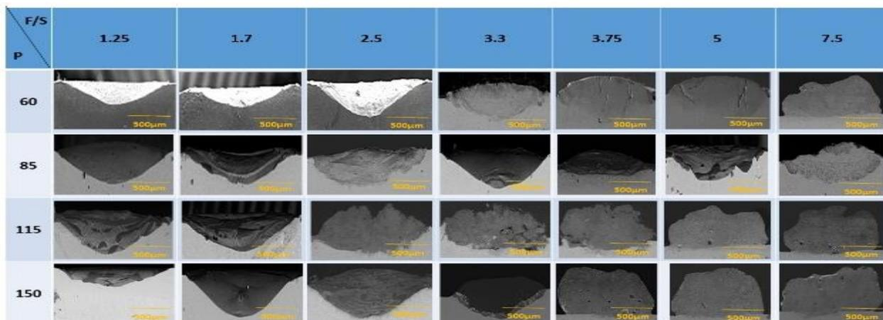
Fig. 2. Cross-sections of single clad in the different samples.
