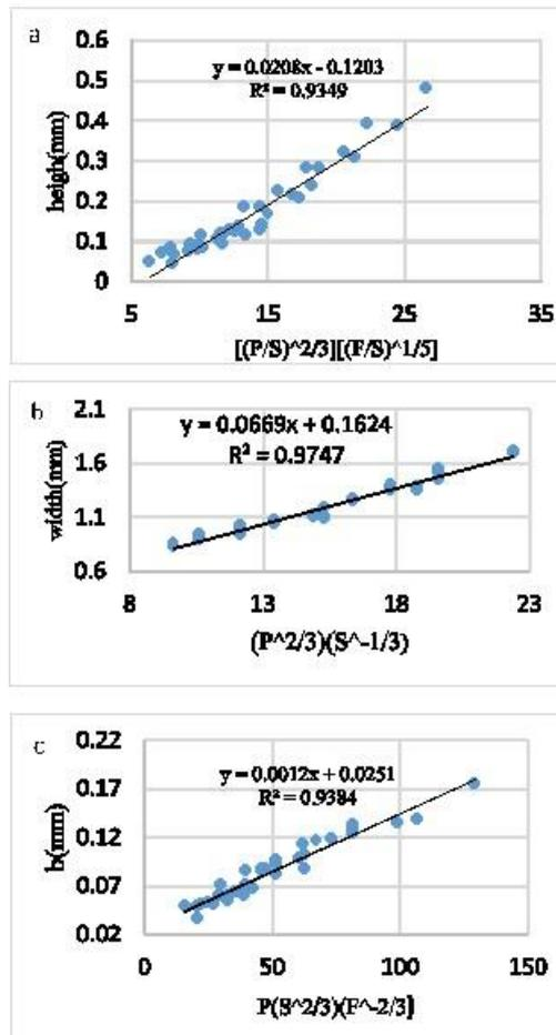
**Fig. 3.** Combined process parameters for three geometrical features of a) height, b) width and c) penetration depth.
