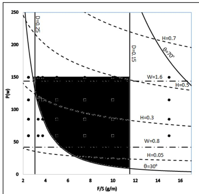
Fig. 5. Processing window for laser cladding of Al powder on In 738.
