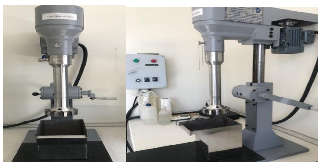
Fig. 1. Images of laboratory flotation machine.
