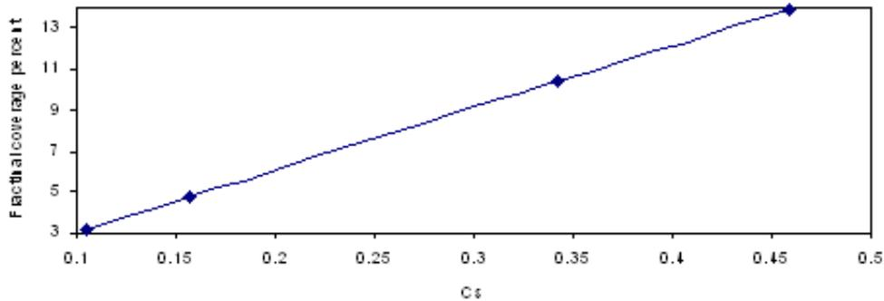
Fig. 4. The fractional coverage surface HEMA versus concentration of protein on the surface at pH 7.2 and 22°C.
