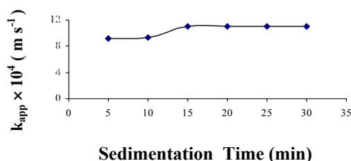
**Fig.10.** Plot of pseudo- first order constant against sedimentation time with Fe/Fe electrode pair.  $C_{0[AY23]} = 40 \text{ mg l}^{-1}$ ,  $C_{NaCl} = 400 \text{ mg l}^{-1}$ ,  $t_{elec.} = 5 \text{ min}$ ,  $d = 1.5 \text{ cm}$ ,  $T = 295 \text{ K}$ .
