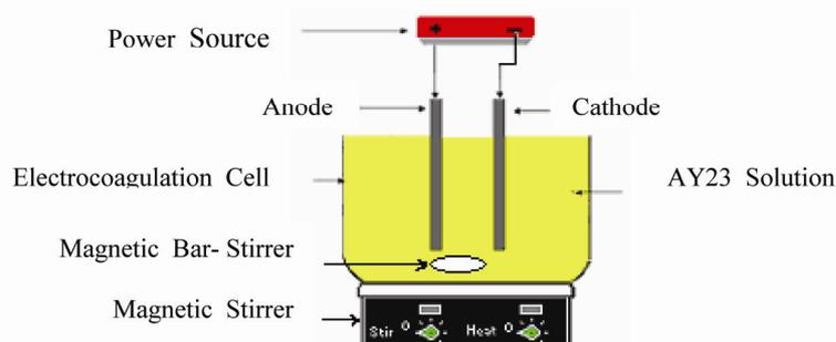
Fig.1. The experimental EC reactor.
