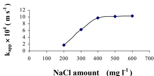
**Fig.4.** Effect of NaCl amount on the pseudo- first order rate constant with Fe/Fe electrode pair.  $C_{0[AY23]} = 40 \text{ mg l}^{-1}$ ,  $t_{elec.} = 5 \text{ min}$ ,  $[i] = 120 \text{ A m}^{-2}$ ,  $d = 1.5 \text{ cm}$ , sedimentation time = 20 min,  $T = 295 \text{ K}$ .
