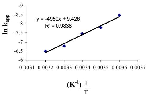
**Fig.6.** Effect of reaction temperature on the pseudo- first order rate constant with Fe / Fe electrode pair.  $C_{0[AY23]} = 40 \text{ mg l}^{-1}$ ,  $C_{NaCl} = 400 \text{ mg l}^{-1}$ ,  $t_{elec.} = 5 \text{ min}$ ,  $[i] = 120 \text{ A m}^{-2}$ ,  $d = 1.5 \text{ cm}$ , sedimentation time = 20 min,  $T = 295 \text{ K}$ .
