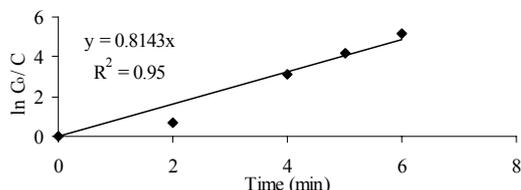
**Fig.2.** Logarithm of normalized AY23 concentration as a function of electrolysis time with Fe / Fe electrode pair.  $C_{0[AY23]} = 40 \text{ mg l}^{-1}$ ,  $C_{NaCl} = 400 \text{ mg l}^{-1}$ ,  $[i] = 120 \text{ A m}^{-2}$ ,  $d = 1.5 \text{ cm}$ , sedimentation time = 20 min,  $T = 295 \text{ K}$ .
