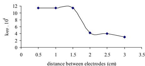
**Fig.9.** Plot of pseudo- first order constant against distance between the electrodes with Fe/Fe electrode pair.  $C_{0[AY23]} = 40 \text{ mg l}^{-1}$ ,  $C_{NaCl} = 400 \text{ mg l}^{-1}$ ,  $t_{elec.} = 5 \text{ min}$ , sedimentation time = 20 min,  $T = 295 \text{ K}$ .
