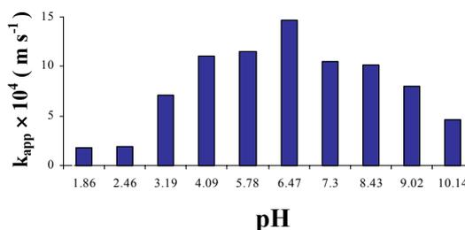
**Fig.8.** Effect of pH on the pseudo- first order rate constant with Fe/Fe electrode pair.  $C_{0[AY23]} = 40 \text{ mg l}^{-1}$ ,  $C_{NaCl} = 400 \text{ mg l}^{-1}$ ,  $t_{elec.} = 5 \text{ min}$ ,  $[i] = 120 \text{ A m}^{-2}$ ,  $d = 1.5 \text{ cm}$ , sedimentation time = 20 min,  $T = 295 \text{ K}$ .
