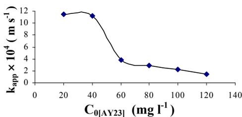
**Fig.3.** Plot of pseudo-first order rate constant against initial concentration of AY23 with Fe / Fe electrode pair.  $C_{NaCl} = 400 \text{ mg l}^{-1}$ ,  $t_{elec.} = 5 \text{ min}$ ,  $[i] = 120 \text{ A m}^{-2}$ ,  $d = 1.5 \text{ cm}$ , sedimentation time = 20 min,  $T = 295 \text{ K}$ .
