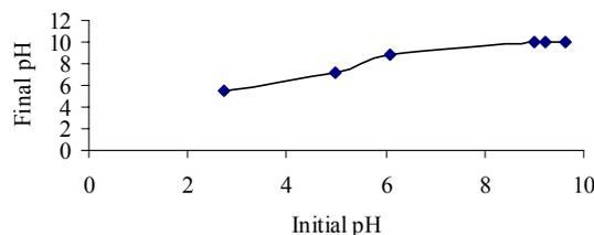
**Fig.7.** The pH change of AY23 solution after electrocoagulation as a function of initial pH with Fe/Fe electrode pair.  $C_{0[AY23]} = 40 \text{ mg l}^{-1}$ ,  $C_{NaCl} = 400 \text{ mg l}^{-1}$ ,  $t_{elec.} = 5 \text{ min}$ ,  $[i] = 120 \text{ A m}^{-2}$ ,  $d = 1.5 \text{ cm}$ , sedimentation time = 20 min,  $T = 295 \text{ K}$ .
