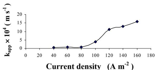
**Fig.5.** Plot of pseudo- first order constant against current density with Fe / Fe electrode pair.  $C_{0[AY23]} = 40 \text{ mg l}^{-1}$ ,  $C_{NaCl} = 400 \text{ mg l}^{-1}$ ,  $t_{elec.} = 5 \text{ min}$ ,  $d = 1.5 \text{ cm}$ , sedimentation time = 20 min,  $T = 295 \text{ K}$ .
