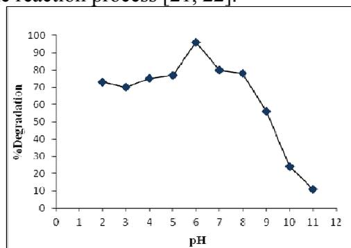
**Fig. 7.** Effect of  $pH$  on the photodegradation efficiency.
