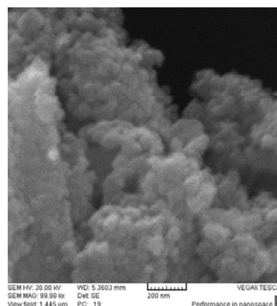
Fig. 2. SEM image of CuO/ZnO nanoparticles.
