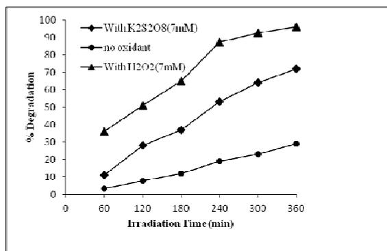
**Fig. 6.** Effect of electron acceptors on the photodegradation efficiency.
