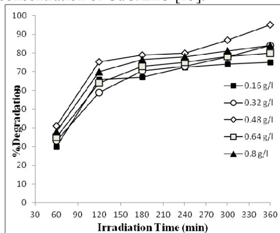
**Fig. 4.** Effect of the amount of ZnO/CuO on the photodegradation efficiency
