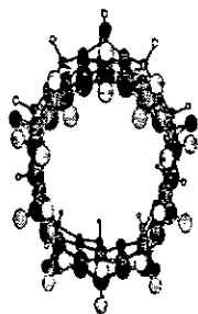
Fig. 2. Zigzag carbon nanotube (10-0) with five oxygen atoms.
